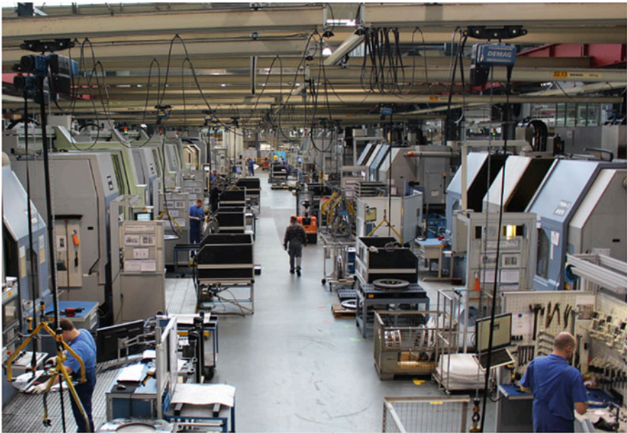
Fig. 10.4 Machine-centers for turning, milling, and drilling (© Knorr-Bremse Berlin SfS GmbH)
